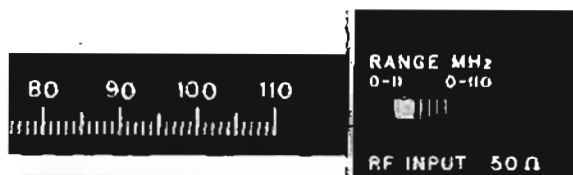
Figure 1. Expanded Dial Scale. When the Expanded Dial Scale is selected the 0 - 110 MHz dial becomes 0 - 11 MHz. Dial resolution is 200 kHz; tuning resolution much easier.
