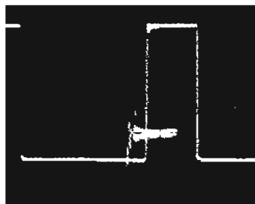
Double exposure showing 5-div pulse on upper waveform, and the same pulse expanded 10 X to view small perturbation on the top.
