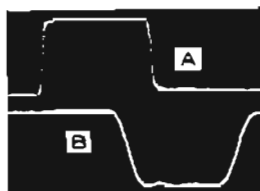
Figure 2. (A) Input Pulse to HP 462A (5 mV peak to peak). (B) Output Pulse of HP 462A (500 mV peak to peak). Gain control is set in 40 dB position. Sweep speed is 5 ns/cm.
